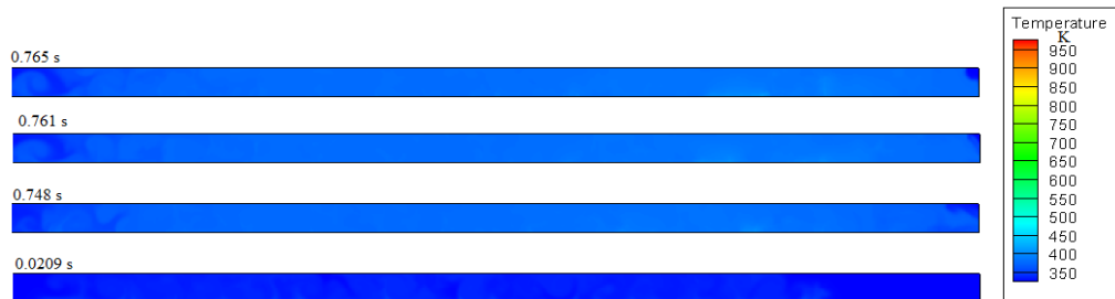
Figure 7. Two-phase flow in 800 μm height microchannel at 1.311 \times 10^{-6} kg/s as a mass flow rate and 500KW/m as a heat flux
