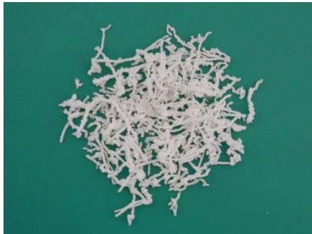
Fig # 1: PMMA sheet drilled threads
