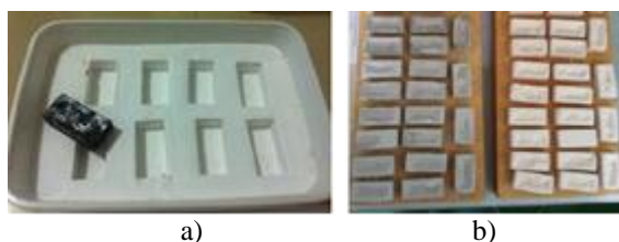
Fig (1) a) plaster mold for porcelain samples preparation and b) porcelain clay products after casting.
