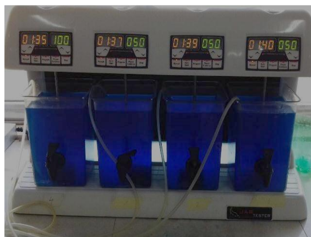
Figure.1: Jar Test apparatus
