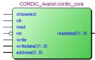
Fig (3) The functional block diagram of the custom component
