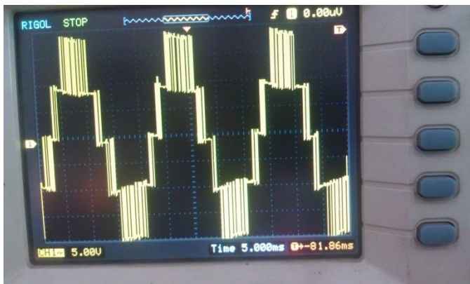
Fig 12: Output Line-to-line voltage over SVM control
