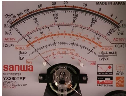
Figure 1. A portion of an analog multimeter, the Sanwa YX360TRF
