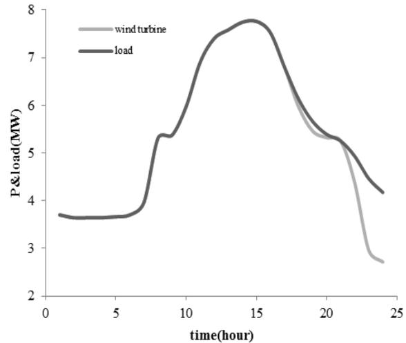
Figure 7 Supply WT and load profile
