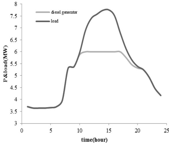
Figure 6 Supply diesel generator and load profile
