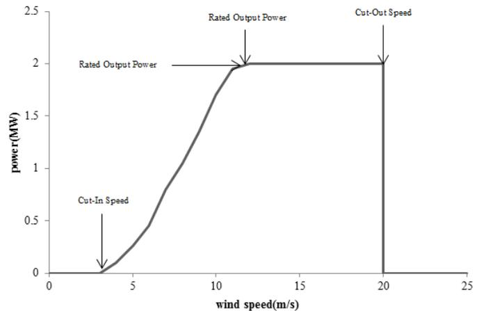
Figure 3 WT p-v curve [12]
