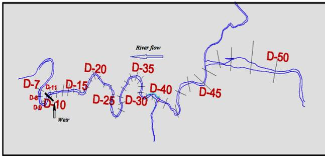
**Fig. 1: Schematic Diagram showing the Cross Sections Locations used for the delta modeling.**
