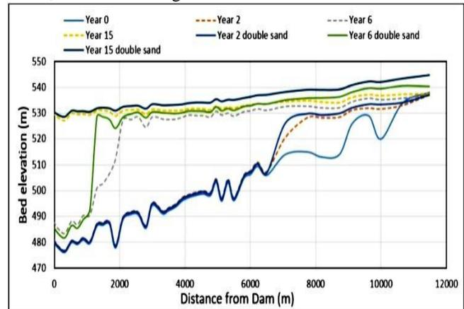
**Fig.16. Comparison of longitudinal profiles for Test 2 and Test 8**
