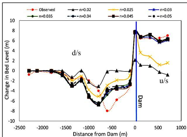
Fig. 8. Change in river bed level for different values of “n”
