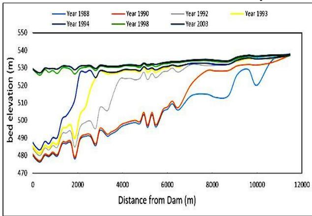
**Fig.13. Longitudinal Bed Profiles Along the Reservoir for the Flow Series with a Large Event (Test 2)**
