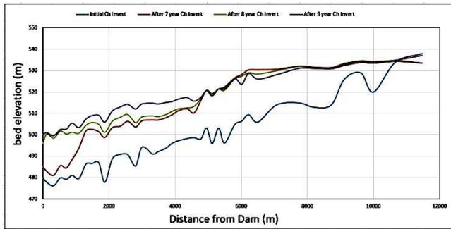
**Fig. 19: Bed profile after 7th, 8th and 9th years flushing**
