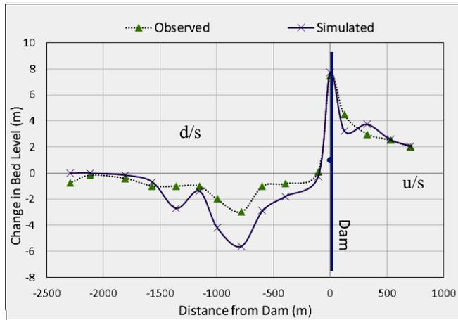
Fig. 11. Change in river bed level under 1 gate opening condition
