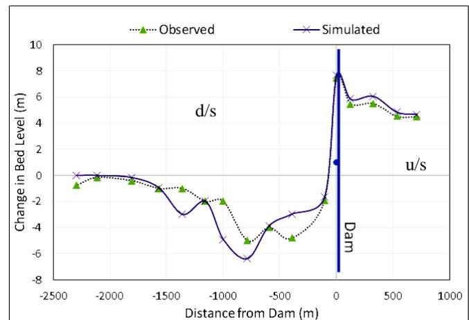
Fig. 10. Change in river bed level under 3 gate opening condition
