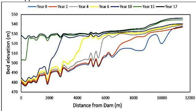
**Fig. 14. Longitudinal Bed Profiles along the Reservoir (Test 5)**
