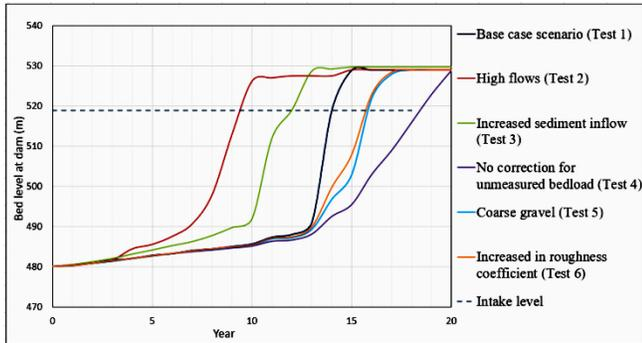
Fig. 17. A comparison of bed levels at dam with the level of intakes (Tests 1-6)
