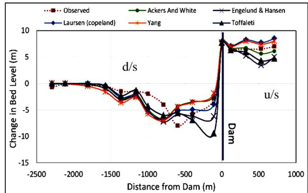
Fig. 9. Change in river bed level for different sediment transport functions.
