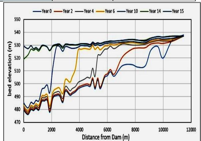
Fig.12. Longitudinal Bed Profiles along the Reservoir for the Base Case Scenario (Test 1)
