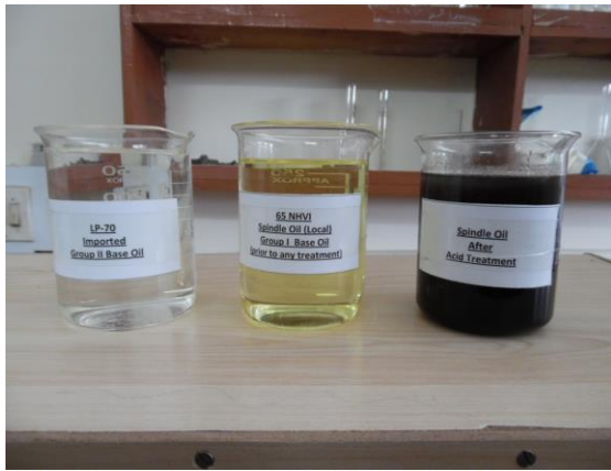
Figure 3.1. Color comparison of Group II base oil (Imported), Group I base oil (Local) and Group I base oil (after acid treatment)
