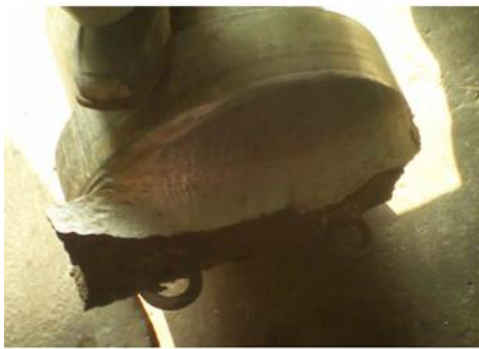
Figure 6: Photograph of Actual Broken Blade
