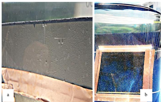
Fig. 8 - Bubbling experiment of artificial leaf B (a) H 2 -Bubbles formation from the p-side of the Solar Cell. (b) O 2 -Bubbles formation from the n-side of the Solar Cell.
