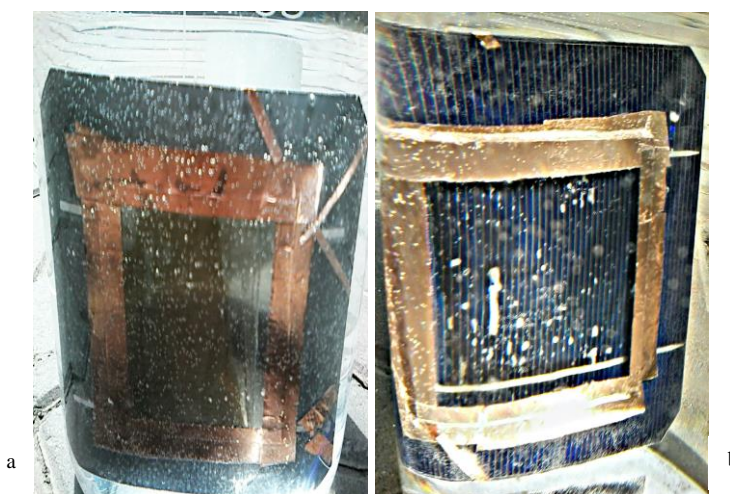
Fig. 9 - Bubbling experiment (a) Enhanced H 2 -Bubbles formation from the p-side of the Solar Cell, (b) Enhanced O 2 -Bubbles formation from the n-side of the Solar Cell.
