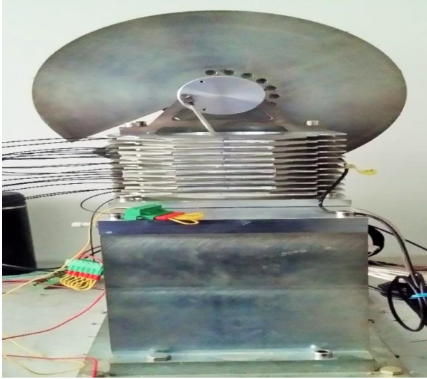
Figure 3 Hardware model of stirling engine (side view)
